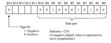
The above diagram shows an example of a 16-bit digital value written from the Q-Series CPU to the digital-to-analogue converter module. Set a digital value of -2048 to +2047 in 16-bit signed binary.
