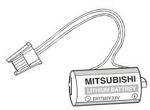
The battery is installed at the bottom side of the Q CPU. During interruption of the power supply the battery can hold the data of the program memory , the built-in RAM and the clock for several thousand hours. However, this time depends on the type of CPU.
