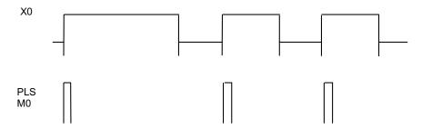
From the above waveforms, it can be seen that each time Input X0 operates, the Instruction PLS M0 will be executed and the normally open contact of M0 will momentarily close, hence causing the Counter C0 to be reset to zero.
