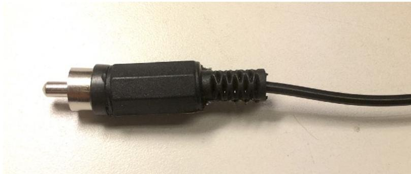
Slide the plug cover back over the plug, and carefully thread it back on. If you like, you can tie a loop knot in the other end of the antenna to make it convenient to hang the end of the antenna on something.
