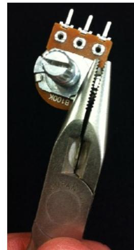
When soldering the pots to the PCB, make sure to leave just a tiny gap between the shoulders of the potentiometer pins and the PCB. If you jam the pot down tight against the PCB, over time the shoulders of the pins might wear thru the soldermask and short against the PCB traces.
