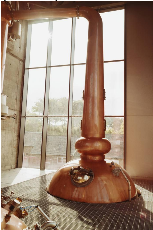
One of the two state-of-the-art copper pot stills in the Lighthouse © Benjamin McMahon
