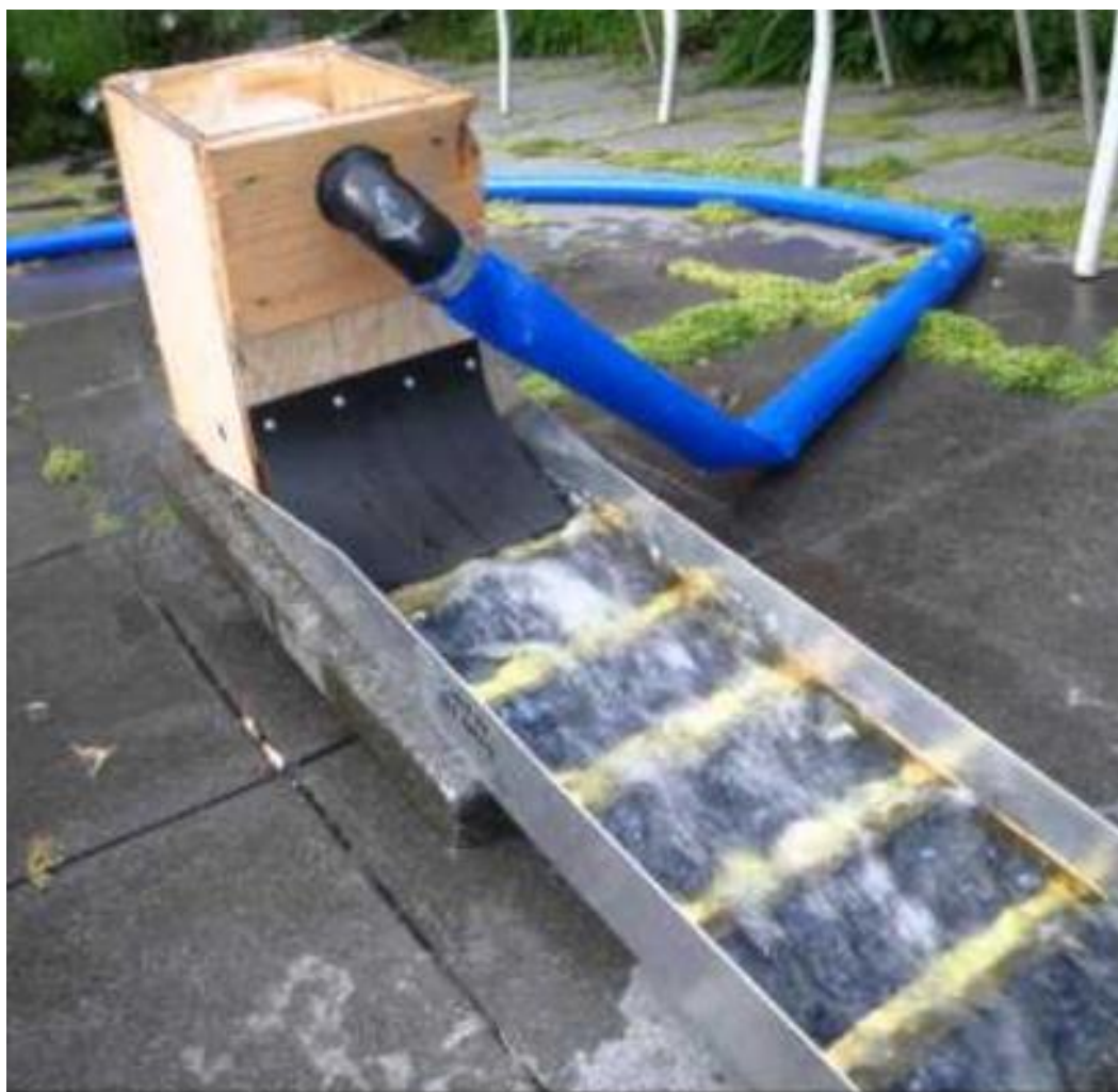
Figure 10. Showing lay flat pressure hose kinking under high flow.
