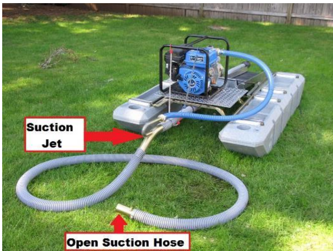
Figure 7. Dredge showing pressure hose (blue), suction jet, and larger open suction hose.
