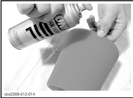
TYPICAL - OIL THE FOAM FILTER
