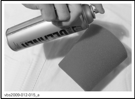
TYPICAL - SPRAY THE FOAM FILTER
