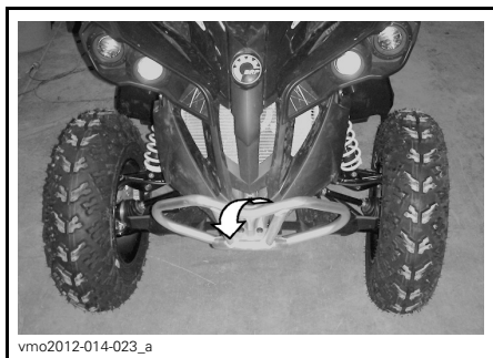
TYPICAL - FRONT TIE-DOWN POINT LOCATION
