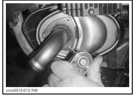
TYPICAL - REMOVE TAIL PIPE
