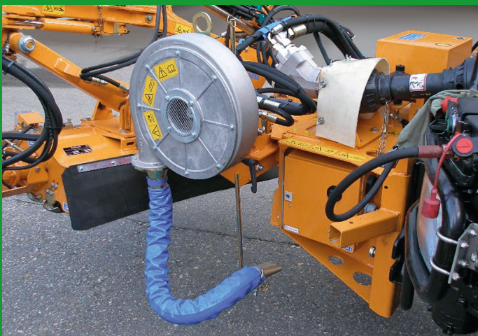
Optional pressure blowing system for effective road cleaning
