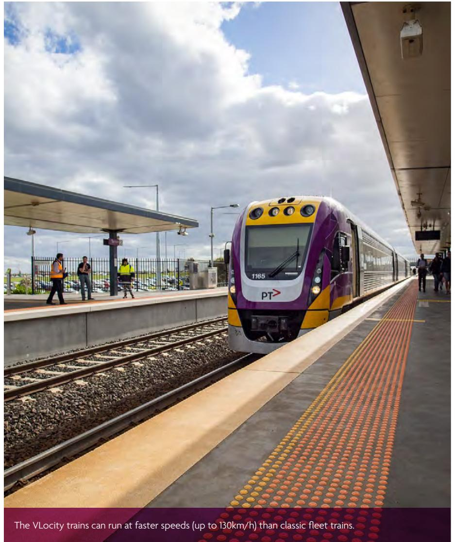
The VLocity trains can run at faster speeds (up to 130km/h) than classic fleet trains.
