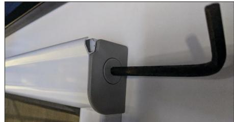
This will unscrew the larger plug and will be already putting more tension on the spring. Usually 3 to 6 turns should add sufficient tension. When enough tension is achieved, while still holding plug against container let it turn clockwise a little and the plug will lock itself back in.
