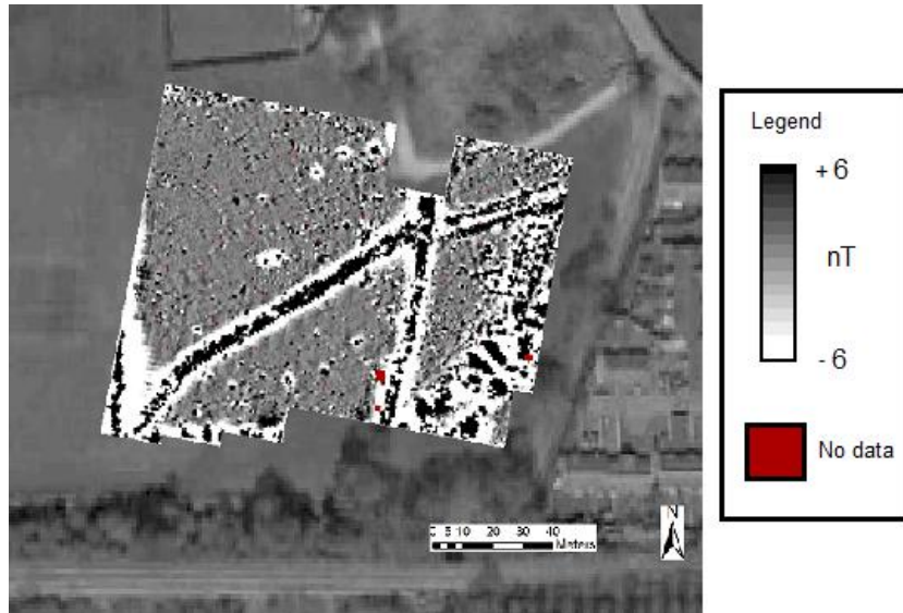
Figure 10: Geophysical Magnetometer Survey Results Area 1, 2016. Magnetometer data greyscale image, Clipped +/- 6nT, Destriped, De-Spiked (Threshold 1.0), Interpolated Vertical. Contains OS data © Crown copyright [and database right] 2016. Contains Image © Google Earth. Image © 2016 Bluesky.
