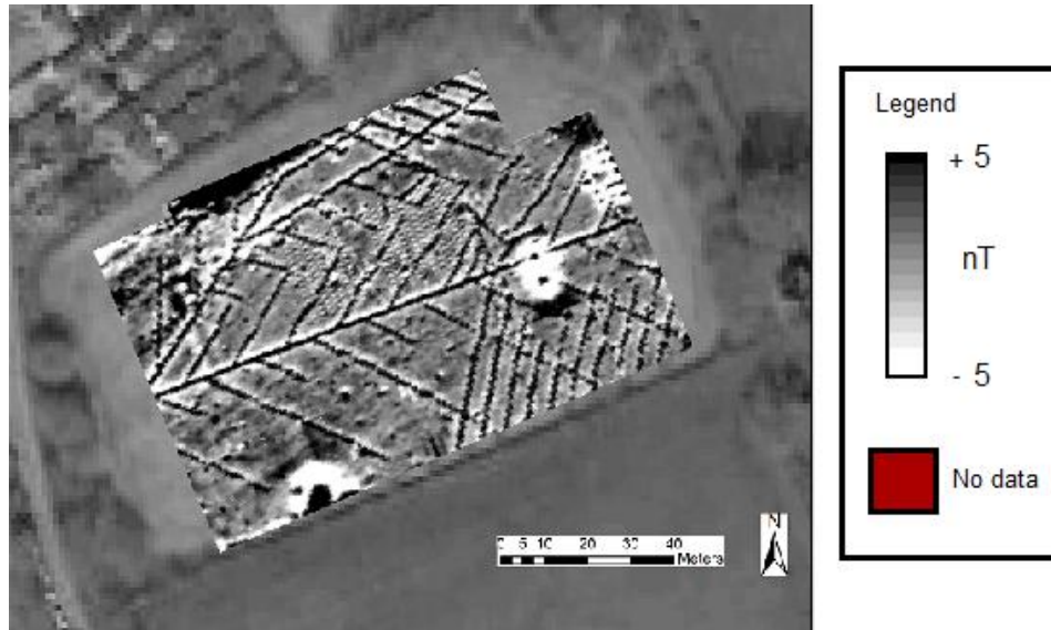
Figure 16: Geophysical Magnetometer Survey Results Area 3, 2016. Magnetometer data greyscale image, Clipped +/- 5NT, Destriped, De-Spiked (Threshold 1.0), Interpolated Vertical. Contains OS data © Crown copyright [and database right] 2016. Contains Image © Google Earth. Image © 2016 Bluesky.
