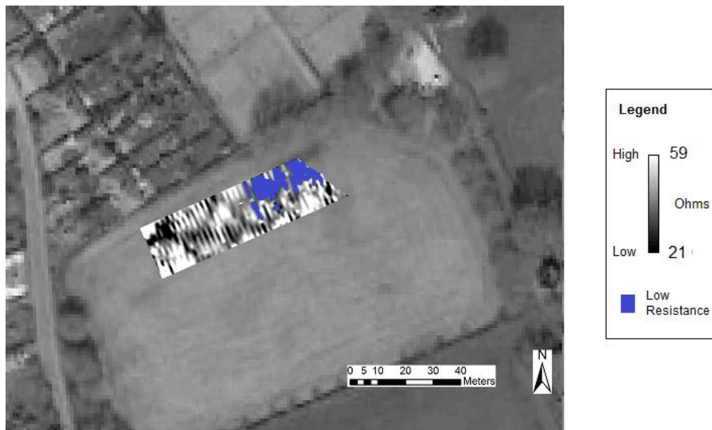
Figure 24: Low resistance Anomaly in Area 6. Contains OS data © Crown copyright [and database right] 2016. Contains Image © Google Earth. Image © 2016 Bluesky.
