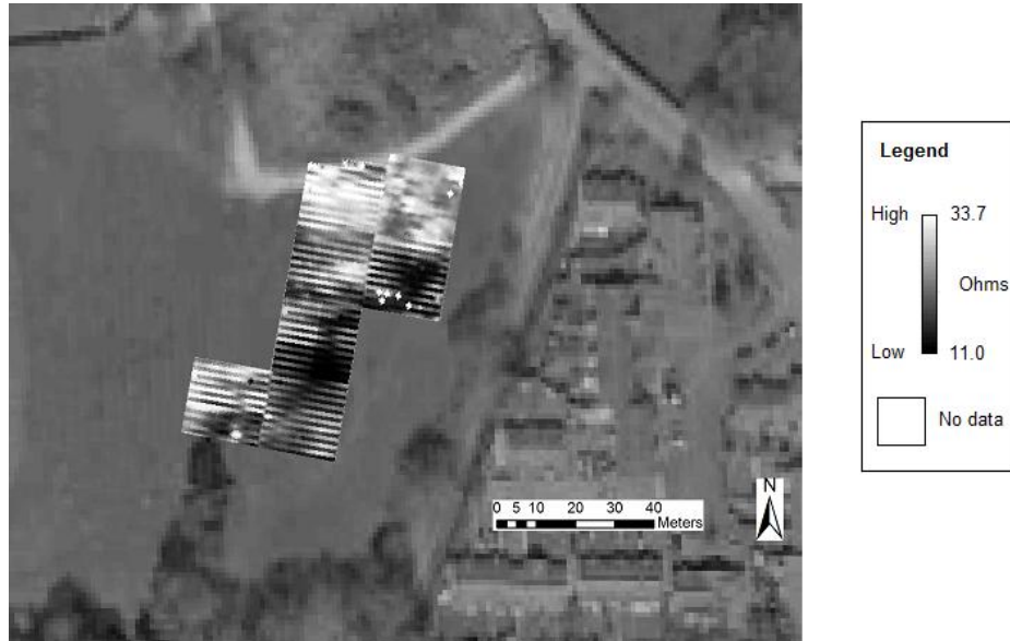
Figure 21: Resistance Survey Results Area 5. Contains OS data © Crown copyright [and database right] 2016. Contains Image © Google Earth. Image © 2016 Bluesky.
