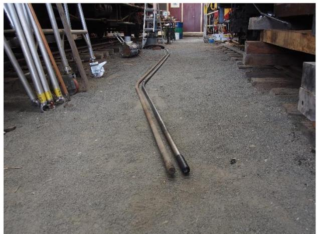
*New truss rod alongside the old. The old one had thread damage and the engineering report indicated the diameter had narrowed too much*
