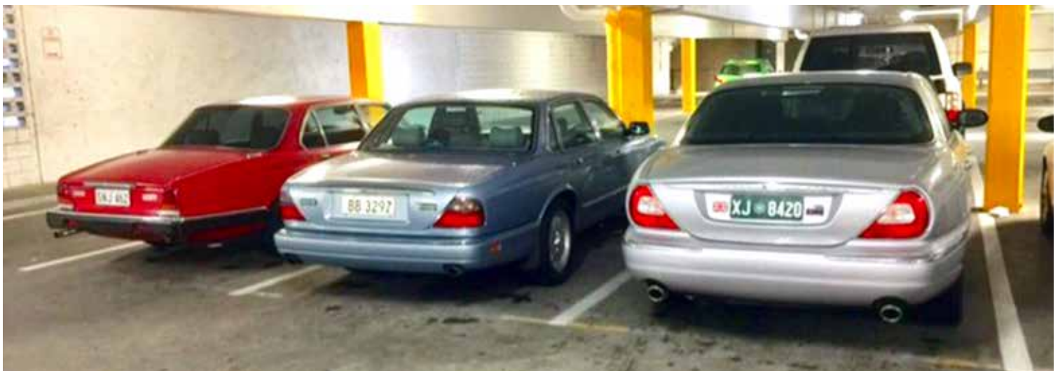
The height evolution of the XJ Jaguar. XJ Series 3 (height 54 in); XJ X300 (height 52.5 in) and Charles X350 (57in).
