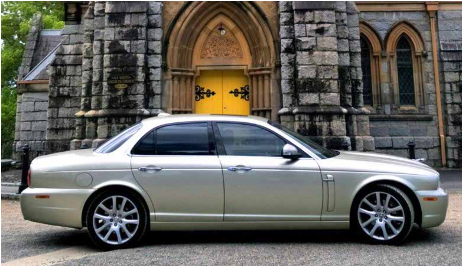
Don & Kathy Tyrrell, 2008 XJ6 X358. The aluminium bodyshell was 40 per cent lighter and 60 percent stiffer than its predecessor despite its increased overall size. A review by Paul Skilleter noted that despite their size, the 'new' XJ's were phenomenally nimble.
