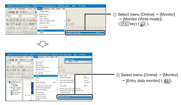
\*The "Entry data monitor" screen can be displayed by selecting [Entry data monitor] with a right click on the ladder screen.
