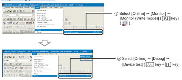
\* The "Device test" screen can be displayed by selecting [Device test] with a right click on the ladder screen.
