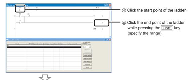
Register devices to the "Entry data monitor" screen.
