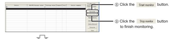
The values of devices and the ON/OFF status of contacts/coils are displayed.
