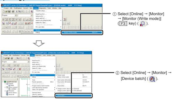
\* The "Device batch monitor" screen can be displayed by selecting [Device batch] with a right click on the ladder screen.
