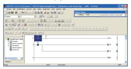
The ON/OFF status of bit devices can be checked on the ladder screen.
