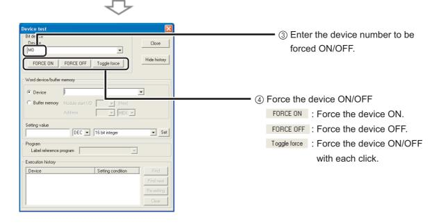
Forcing a bit device ON/OFF with the key operation
