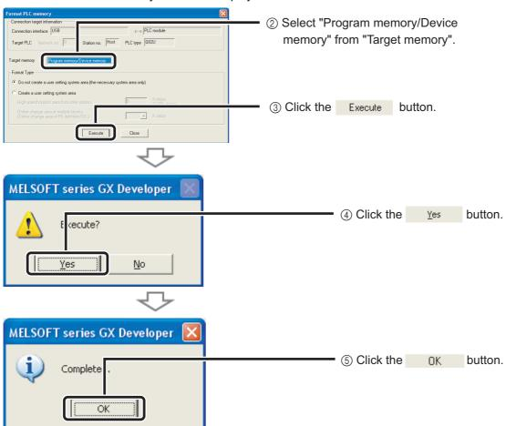
The CPU module format is completed.
