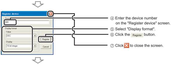
The specified device is registered on the "Entry data monitor" screen.
