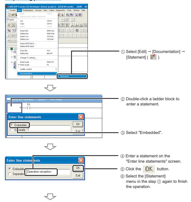
If a statement is entered, a program needs to be "converted" to reflect the input. For details on the conversion, refer to the following page.
