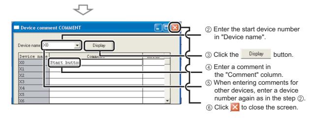
Input operation on the ladder diagram>
