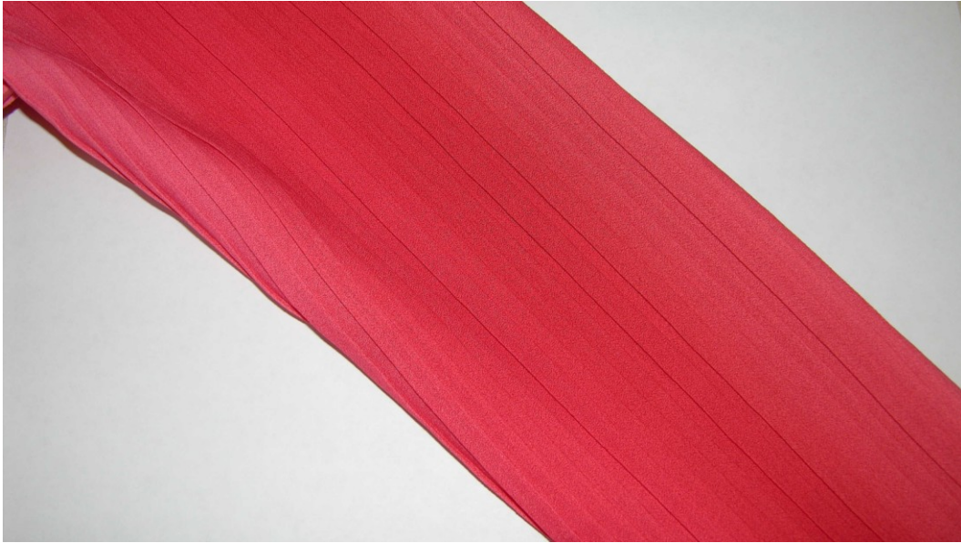
Electric Pleating – the kind of pleating done by an electric pleating machine. Fabrics can be pleated in various widths, sizes and patterns.
