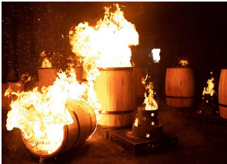
Heat application: Casks are toasted and/or charred using direct flame or a heat element (Photo: Kelvin Cooperage)
