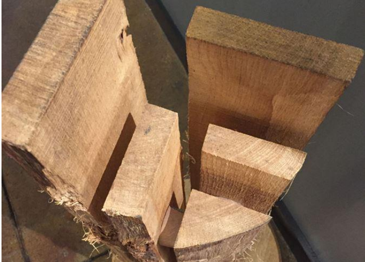
Quarter cut: The heartwood is sawn in a way that makes the cask liquid tight
