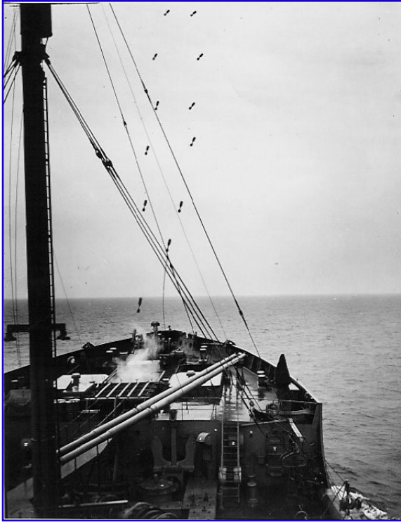
Big Horn's bow-mounted Hedgehog anti-submarine weapons are fired during drills [CDR Douglas L. Jordan (USCGR ret.)]
