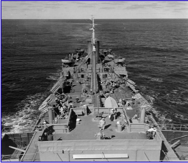
Photo of Big Horn from her bridge showing two of her 4-inch guns hiding behind false bulkheads [CDR Douglas L. Jordan (USCGR ret.)]
