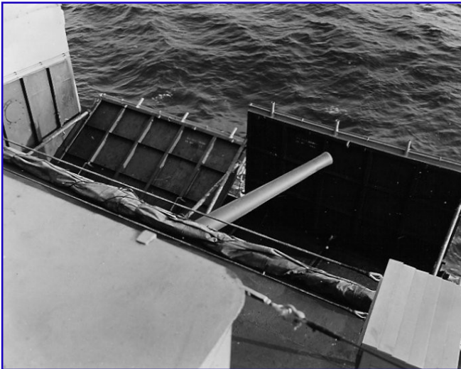
One of Big Horn's 4-inch deck guns is un-masked for gunnery drills [CDR Douglas L. Jordan (USCGR ret.)]
