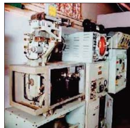
277 radar with covers off the transmitter. (Photo courtesy HMS Collingwood Museum)
