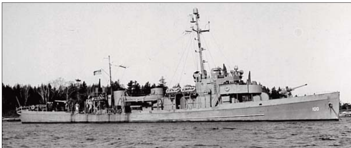
Argo anchored in Love's Cove, near Boothbay, Maine, at the Atlantic war's end in May of 1945. The 165-foot steel cutter was built by John H. Mathis Company at Camden, New Jersey, in 1933. Argo could attain speeds of sixteen knots and was powered by two Winton Model 158 six-cylinder diesel engines, which delivered 1,340 horsepower. (Courtesy of the Winslow Family)
