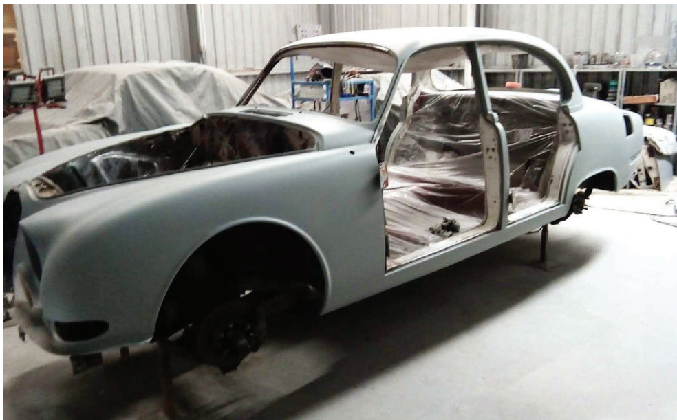
The car was stripped back to bare metal with panels replaced to remove any rust, followed by a repaint and mechanical refurbishment that included a complete engine rebuild.
