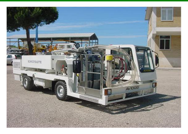
LAVATORY SERVICE ON AVIOGEI SELF – PROPELLED CUSTOM MADE CHASSIS EQUIPPED WITH FRONT LIFTING PLATFORM. HYDRAULICALLY OPERATED. OPERATIVE VACUUM SYSTEM TO OPERATE WITH COMMUTER, N/B, W/B AIRCRAFT
