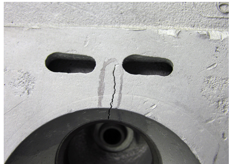
Large crack from combustion chamber to water passage
