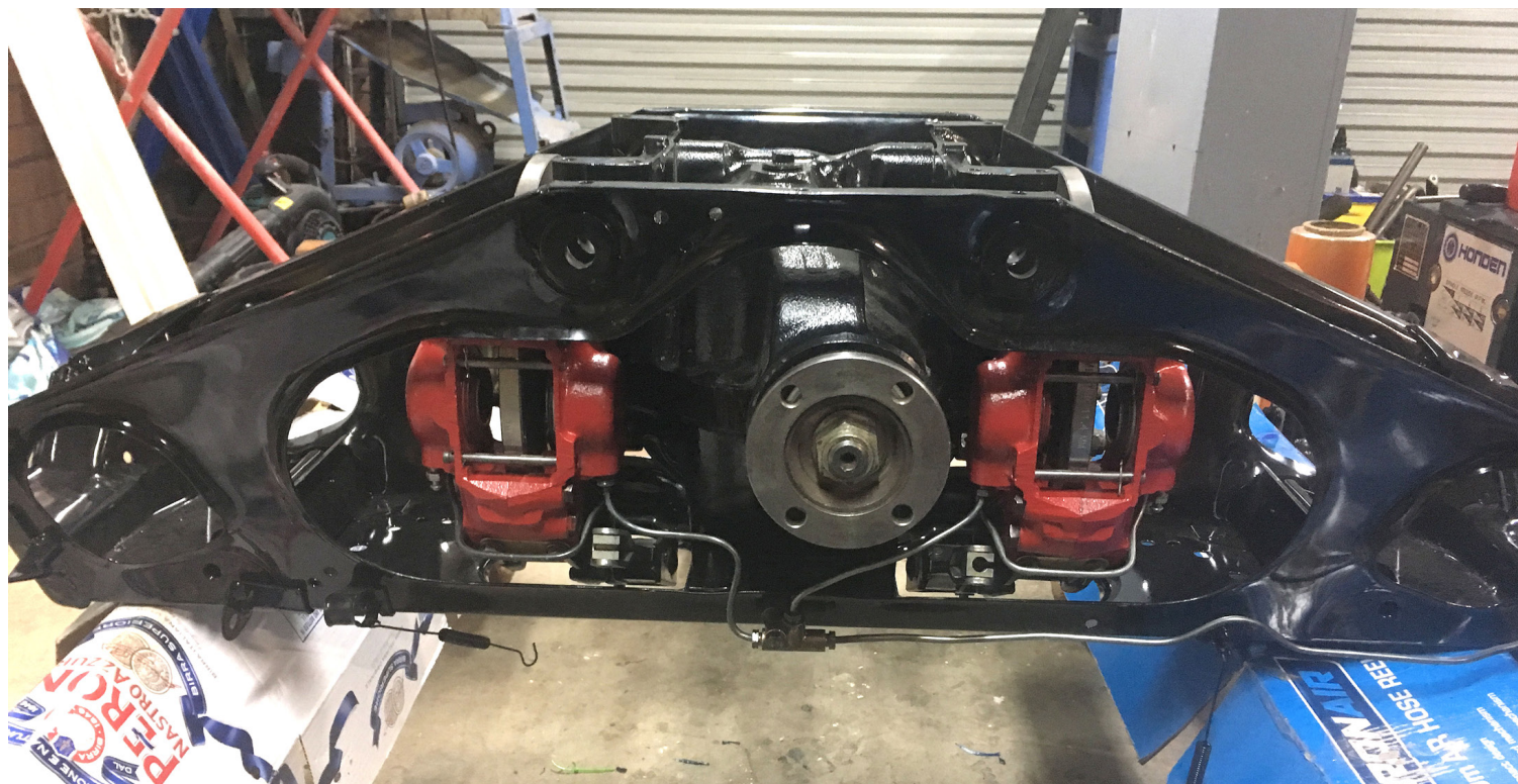
Completed rebuilt rear independent suspension and differential
