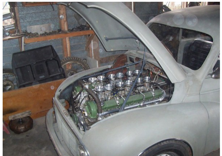
Innocent looking Morris Minor until you lift the bonnet to reveal the V12 Jaguar engine
