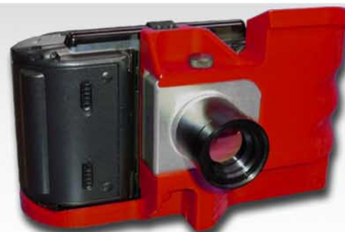
TOP: Rear view of the ICI Prodigy with Sony Micro Computer BOTTOM: Front view of the ICI Prodigy Thermal Imaging System
