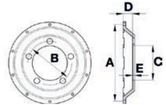
A: Disc Interface PCD B: Stud Bolt Circle C: Center Hole Diameter D: Offset E: Face Thickness
