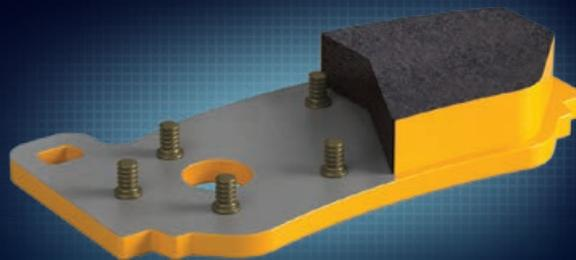
PAGID Racing employs dual retention systems, with an adhesive bond and a patented mechanical system. The mechanical system consists of brass studs that are welded directly to the backplate to ensure a positive retention between pad compound and the backplate. These brass studs are softer than the brake disc (rotor) and wear away as the pad is consumed causing no damage to the disc.
