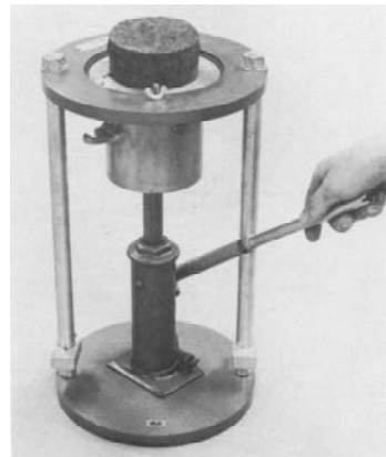
Figure 6.14 Jacking soil out of mould
