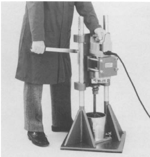
Figure 6.22 Vibrating hammer in supporting frame
