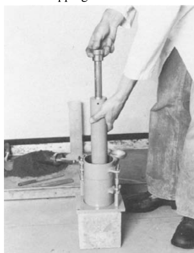
Figure 6.11 Compacting soil into mould
