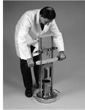
Figure 6.27 Apparatus for moisture condition test (photograph courtesy of ELE International)
