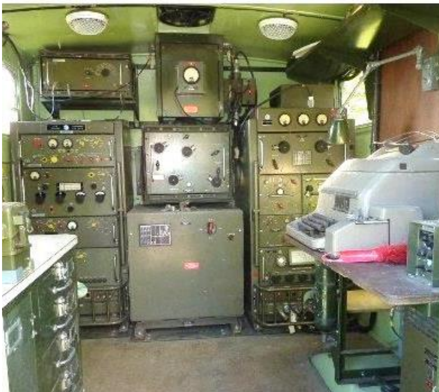
Box body interior showing the D11/R234
