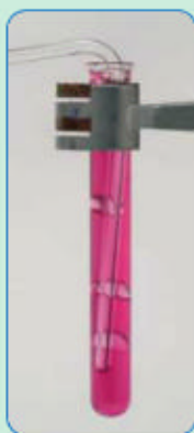
Fig. 26.7 Carbon dioxide dissolves in water to form an acid (carbonic acid). Therefore, the blue litmus indicator turns red when carbon dioxide is bubbled into the water.
