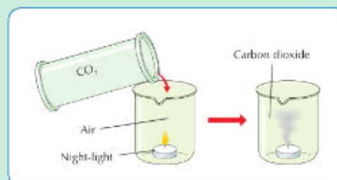
Fig. 26.6 This experiment shows that carbon dioxide is more dense than air. It also shows that carbon dioxide does not allow substances to burn in it. The carbon dioxide flows down and puts out the flame of the night light.
