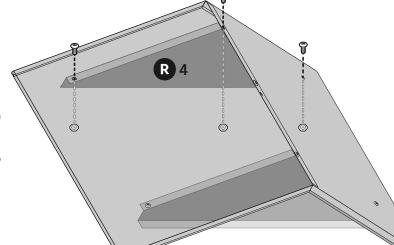
Follow the same method to attach the **R4 roof brace**.
