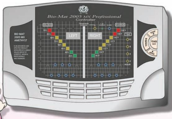
A temperature indicator is shown on the display of the controller. Left side of the display shows a Celsius scale and right side a Fahrenheit scale. In addition, there's also a far infrared ray indicator, an electromagnetic interception indicator, and a built-in alarm system on the controller. On the right side, there's a power switch, temperature control buttons and time control buttons.
