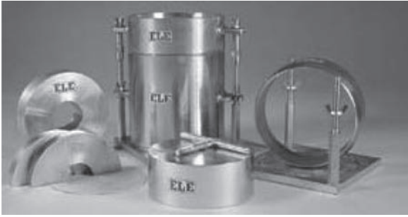
Figure 11.17 CBR mould, fittings and accessories (ASTM type)
