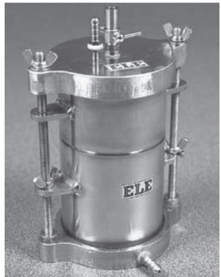
Figure 10.42 Apparatus for falling head permeability test in BS compaction mould
