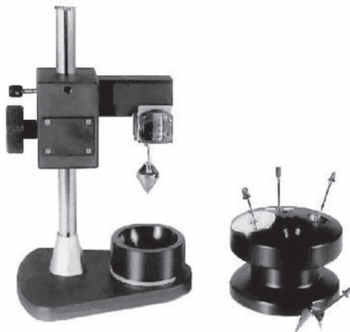
Figure 12.69 Fall cone apparatus (photograph courtesy of Geonor AS)
