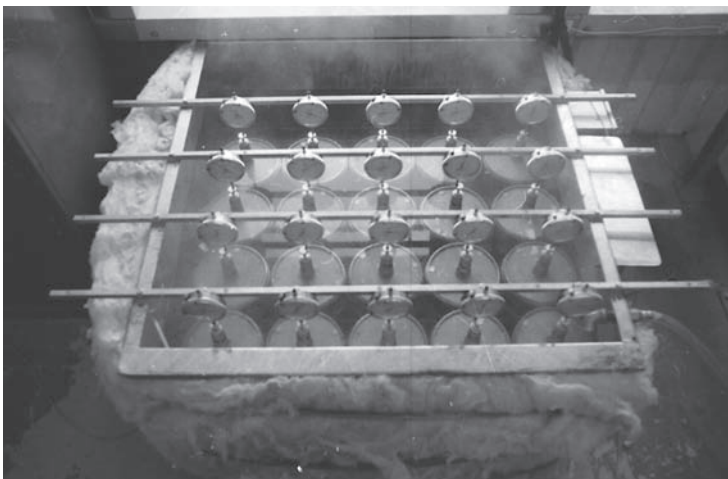
Fig 14.45 Accelerated expansion tests on multiple samples of slag
