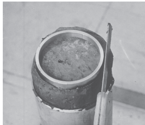
Figure 9.20 Cutting soil from around ring as it is pushed into sample
