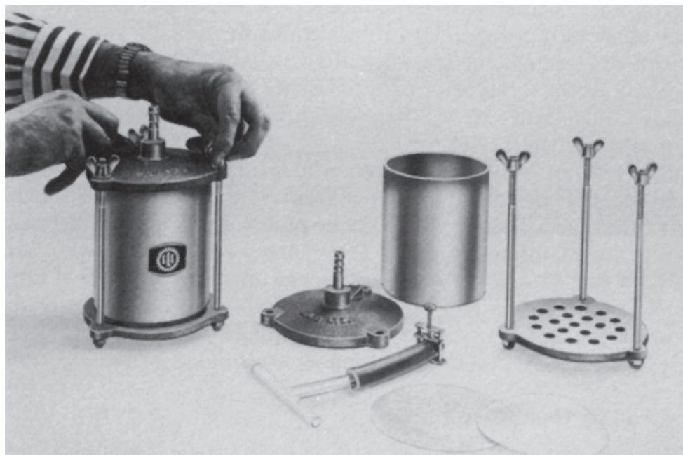
Figure 10.37 Permeameter cell 100 mm diameter and components for falling head test
