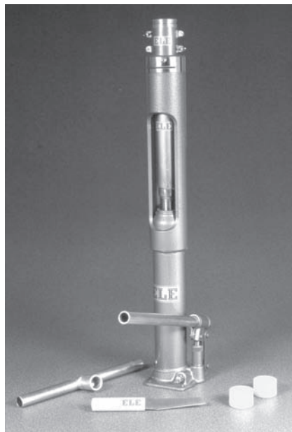
Figure 9.5 Vertical hydraulic type extruder for 38 mm diameter sample tubes
