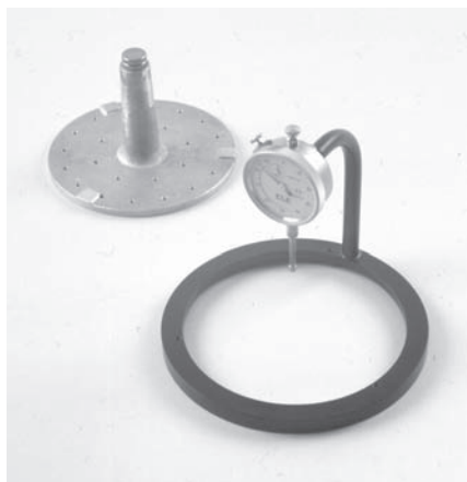
Figure 11.20 Accessories for measurement of swelling in soaking test
