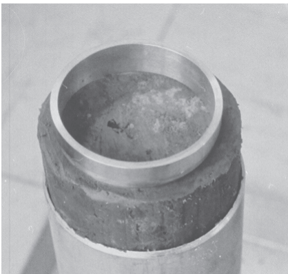
Figure 9.19 Sample partly extruded from U-100 tube for trimming by hand into cutting ring
