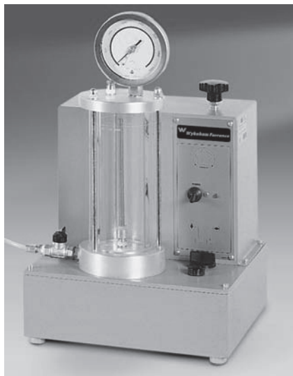
Figure 8.10 Electrically driven oil–water constant pressure system for pressure up to 1700 kPa
