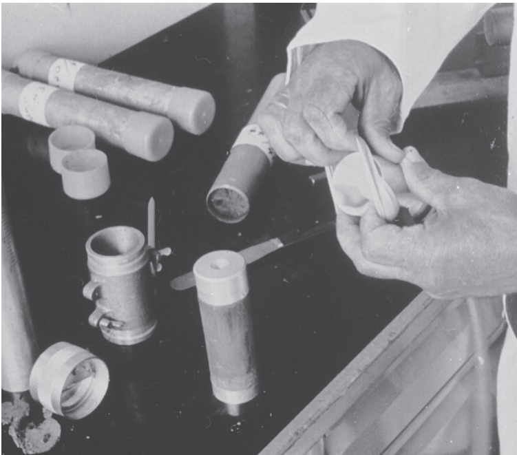
Figure 13.31 Fitting rubber membrane to membrane stretcher
