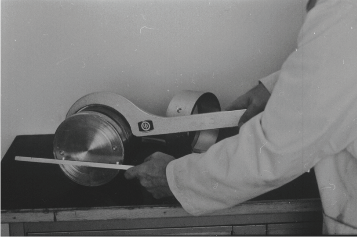
Figure 11.12 Assembling CBR mould and baseplate
