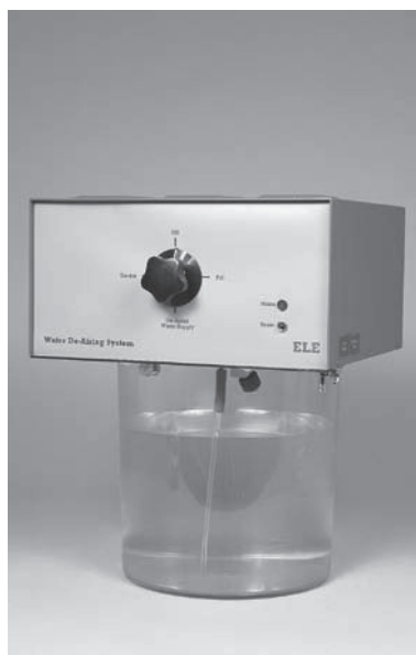
Figure 10.19 (a) Nold de-aerator (photograph courtesy of Geotest Instrument Corp.); (b) automatic de-airing apparatus providing a continuous supply
