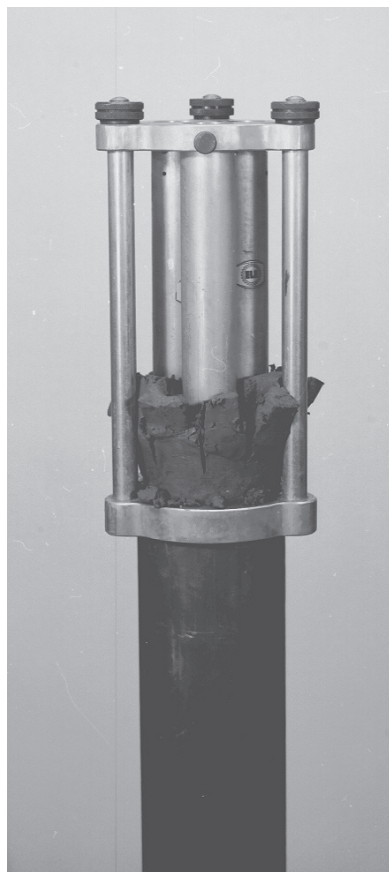
Figure 9.25 Extruding sample from U-100 tube into three 38 mm diameter tubes
