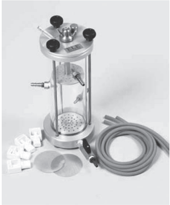
Figure 10.22 75 mm permeameter cell for constant head test
