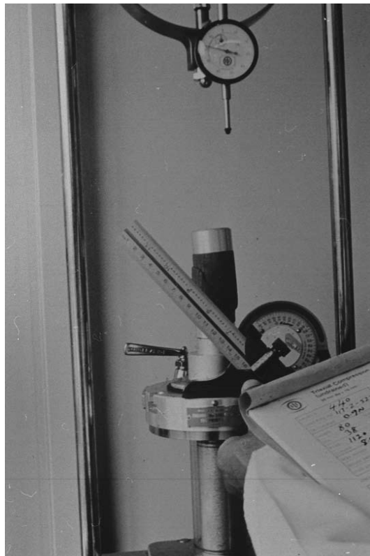
Figure 13.38 Use of engineers protractor to measure inclination of surface at failure
