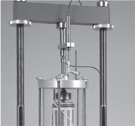
Figure 8.15 Submersible load cell (fitted in a triaxial cell)
