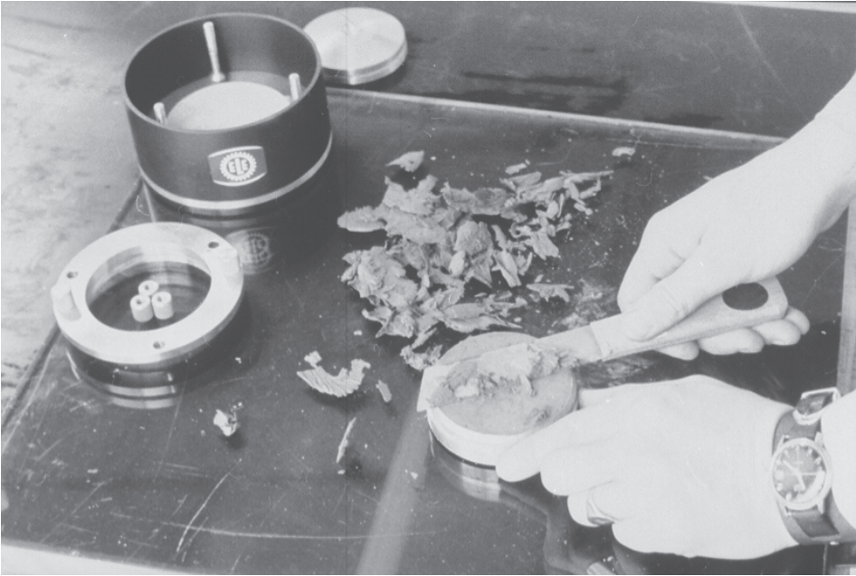
Figure 9.18 Trimming surface of specimen in oedometer ring
