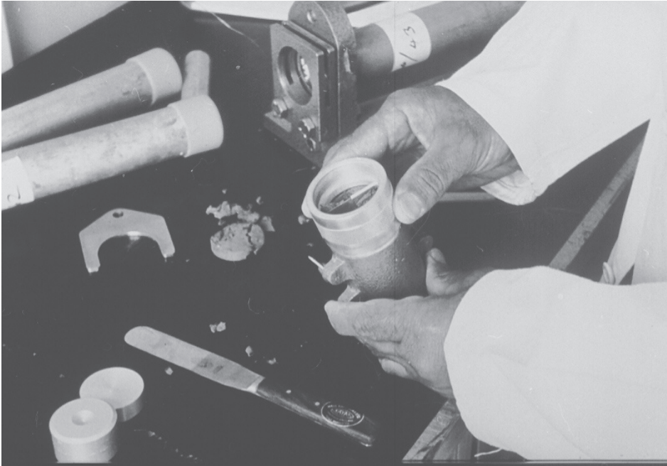
Figure 9.24 Using end trimming tool
