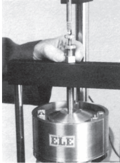
Figure 14.26 Tightening locking nut after adjusting loading stem to bear on top cap
