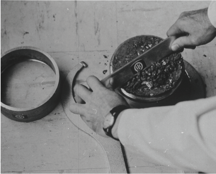
Figure 11.16 Trimming soil surface in CBR mould
