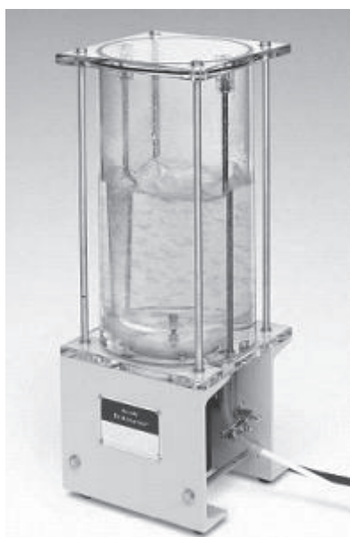
Figure 10.19 (a) Nold de-aerator (photograph courtesy of Geotest Instrument Corp.); (b) automatic de-airing apparatus providing a continuous supply
