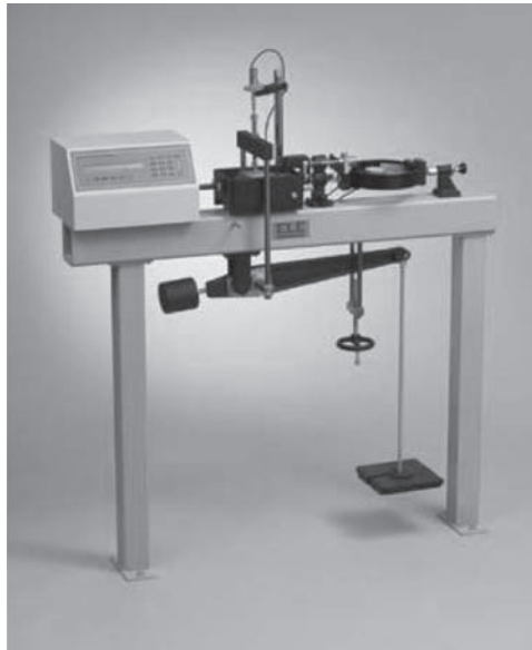
Figure 12.34 Typical shearbox apparatus for 60 \times 60 mm or 100 \times 100 mm specimens
