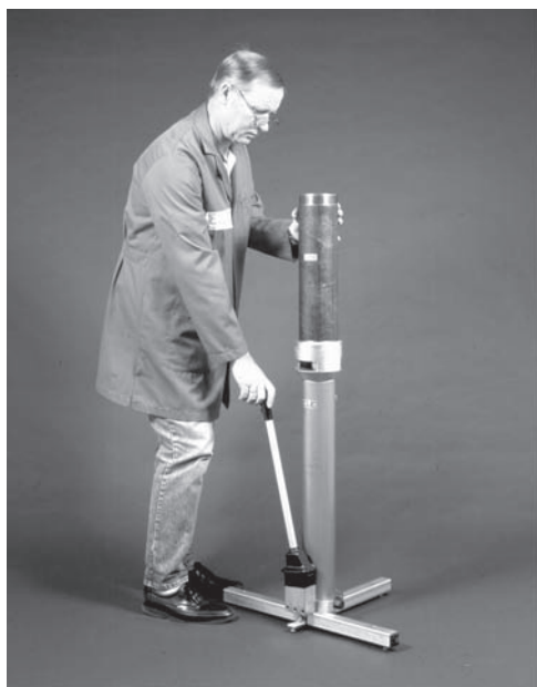
Figure 9.1 Hand-operated hydraulic vertical sample extruder
