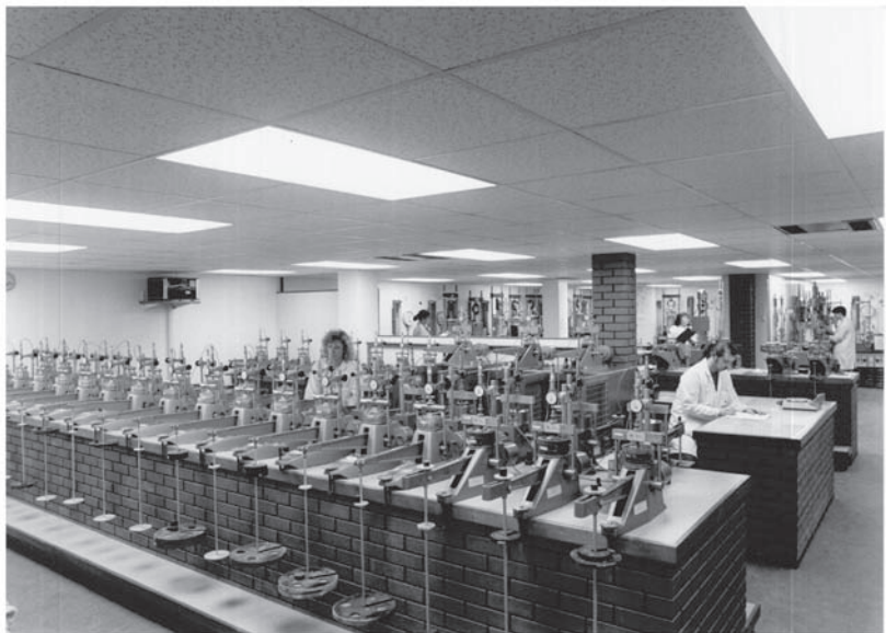
Figure 14.23 Oedometer presses with cells under test (photograph courtesy of Soil Mechanics Ltd)
