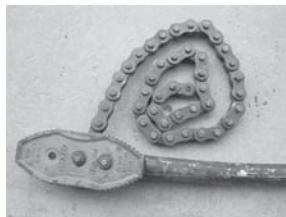
Figure 9.12 Chain wrench, suitable for gripping U-100 tube and end-caps
