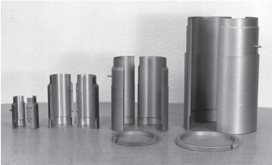
Figure 9.7 Split formers (two segments) for triaxial test specimens of 38, 70, 100, 150 mm diameter
