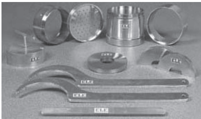
Figure 11.8 CBR mould, fittings and tools for BS tests
