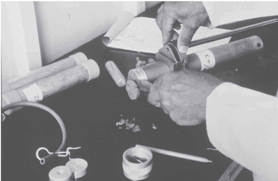
Figure 9.23 Cutting off surplus soil from end of 38 mm diameter specimen in split mould
