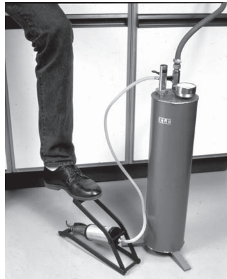
Figure 8.5 Air–water pressure cylinder and foot pump
