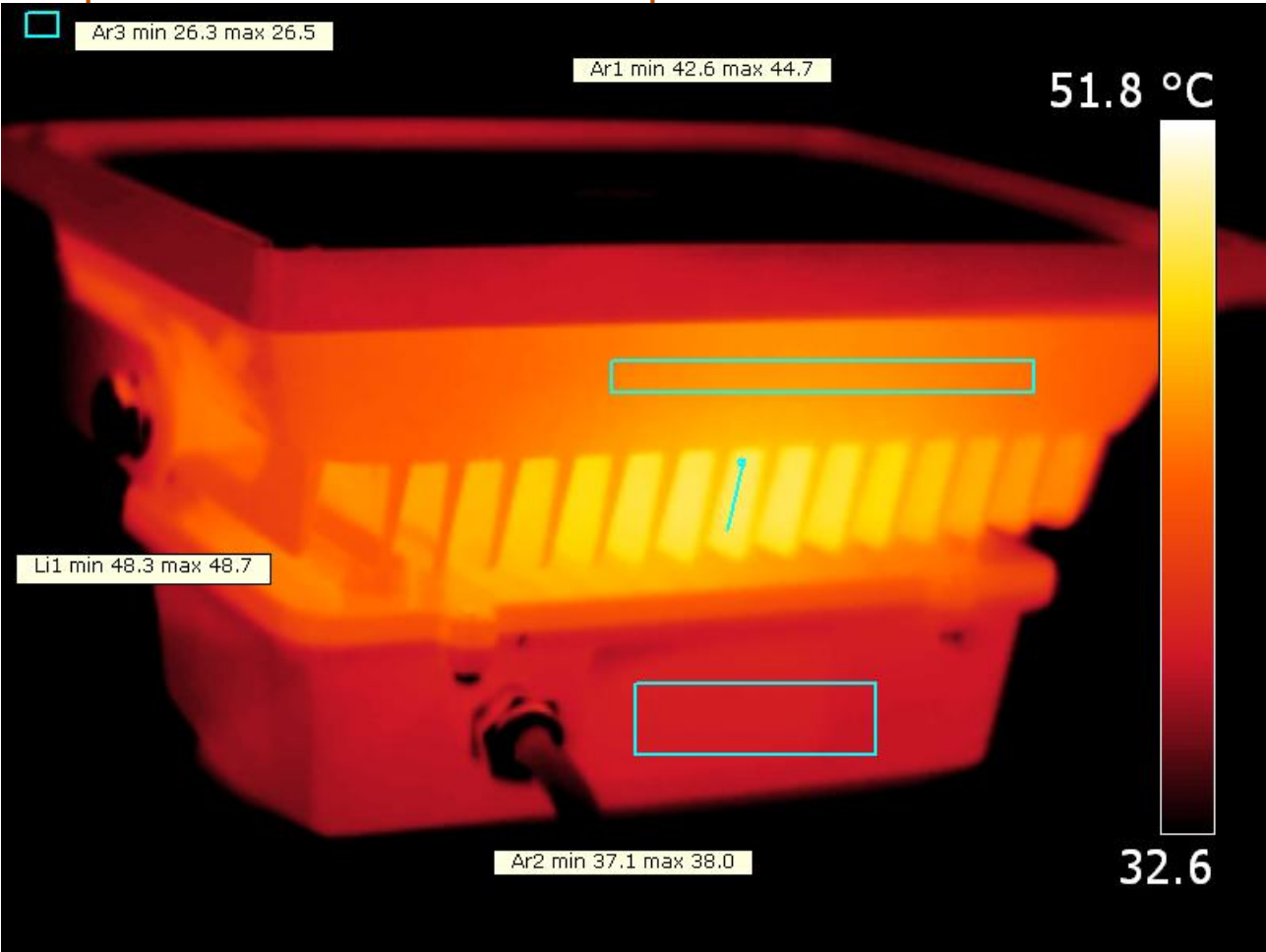
Temp measurement on the side and the bottom, emissivity at 0.95
