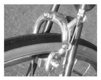
The picture shows the brake of a bicycle. When the cyclist wishes to slow down, she pulls a lever which pushes the rubber brake-pad against the rim of the wheel.
