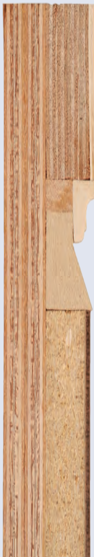
A second doubled layer of bending lauan forms the rails and stiles.
