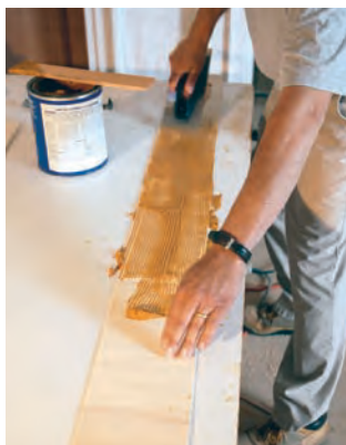
The lauan stiles and rails are covered with 1/8-in. poplar plywood.
