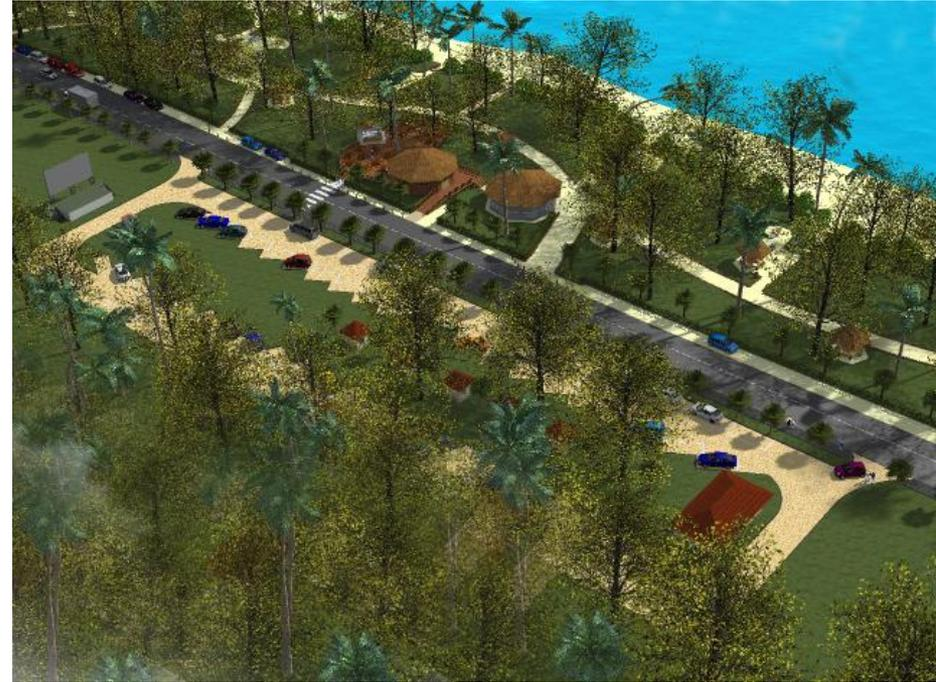
*The proposed car park will be located on the opposite side of the main road as there is sufficient space and appropriate site conditions to accommodate the same. The proposed parking will not be paved, however porous materials such as coarse aggregate may be used. The same will have a designated in and out so as to better control traffic movements along this stretch of road.*
