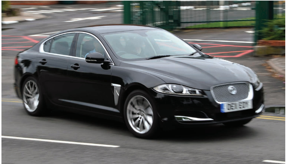
In 2011 the above facelift XF X250.ii, equipped with a 2.2-litre four-cylinder engine completed a 816 mile (1,313km) journey from Castle Bromwich to Munich on a single tank of diesel consuming just 64 litres of fuel to average 4.9 litres/100km. (57.65mpg).
