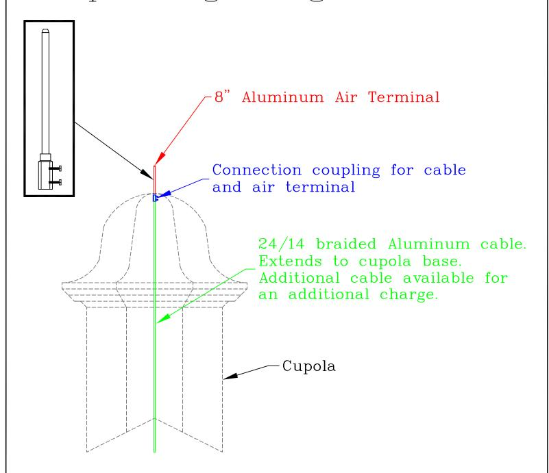
Piedmont Fiberglass or their sub-contractors will not connect the lightning protection. This must be completed by a licensed electrician in compliance with local electrical codes.
