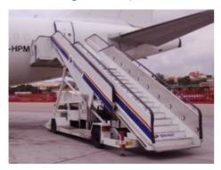
The SmartStep-2 is a self-propelled passenger step designed for universal use with the capability of servicing aircraft with passenger doors from 2.4 to 5.8 meters high. The chassis is purpose-designed specifically for this application.
