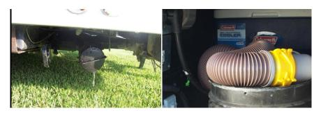
There is also a valve for the shower drain which is closed for travel. It is located on the passenger side of the vehicle just behind the tailpipe, under the RV.
