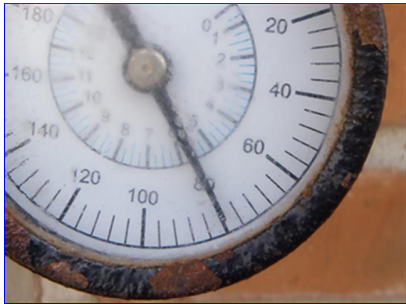
A. Item 1(Picture) Water pressure for the home should be between 40 and 80 psi and was approximately 80 psi at time of inspection.
