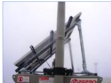
Support Frame Not Grounded
