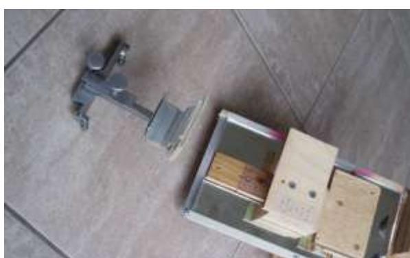
Detail of microscope attachment provision with microscope stage detached from saddle
