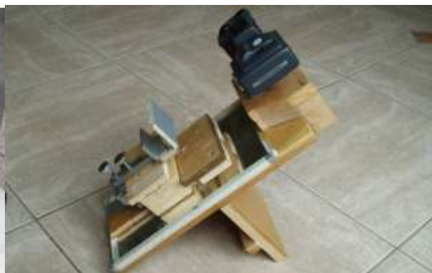
Final developed version of camera/specimen stage using a microscope two axis stage
