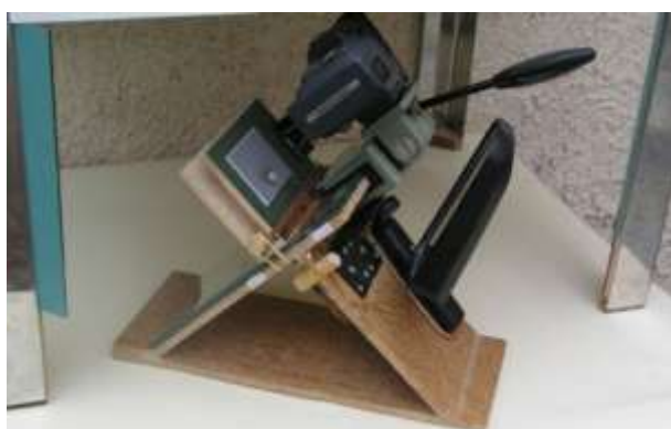
Camera on prototype stage with insect Specimen in position for photography
