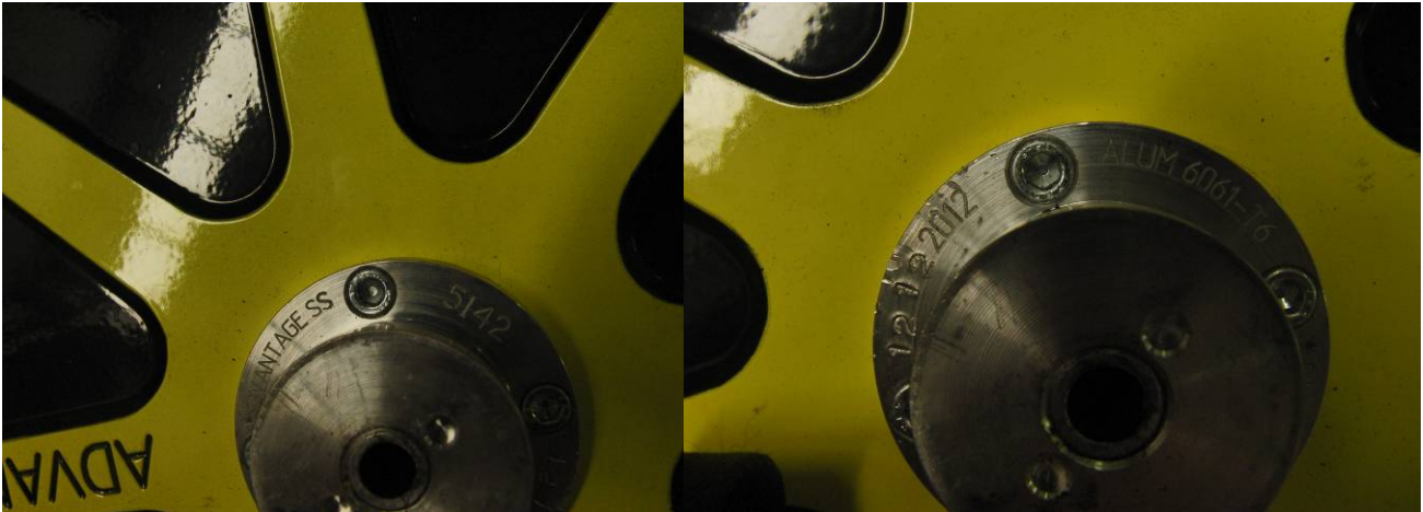
Figure 5 Engraved markings shown on wheels showing manufacturer (Advantage), serial number (5141 & 5142), date of manufacture (2012) and material.
