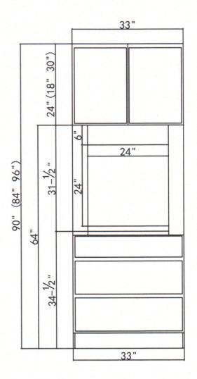
Lower Drawers may be removed to accommodate double ovens. Cabinet can be modified in the field to accept most ovens. Cabinet comes in two pieces; the lower unit is the oven cabinet and a DB33-3(these are sold together) the oven cabinet is 33"w x 31 ½"h the opening is 24" x 24" this can be expanded as needed the total lower unit height is 66", the upper unit is variable to work with your desired height to come out to either 84", 90", or 96" High when combined.
