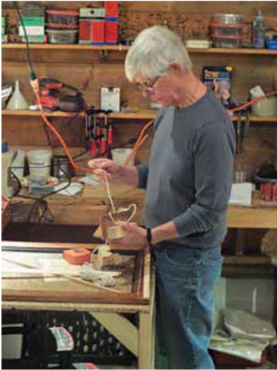
Forsen in his "garage" gallery strings his "corner gizmo" to hold the framefast while glue dries.
