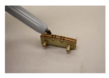
**13.** Assemble the other half of the gluing jig and continue the marked lines across the top.
