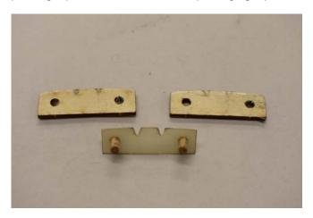
**11. Do Not Glue The Jig Together!** Slip the dowels through the G-10 piece followed by the packing tape lined lite ply part (tape is towards the G-10 part) followed by a non taped lite ply piece.
