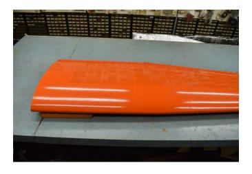
**21.** Using a fine tip marker, add marks onto the wing. See STEP 3 on the drawing.
