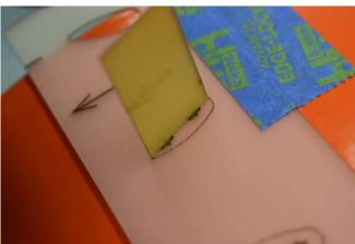
**24.** Remove the template and re-pierce the slots bottoming out the tool onto the sheeting.
