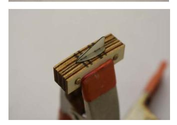
**16.** Using Thick or Medium CA glue with a fine applicator tip run a small bead along both sides then immediately press down on the fin so it conforms to the curvature of the jig. Hold and hit it with an accelerator.
