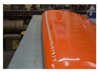
**30.** !/4" balsa protectors are provided. Check fit and chamfer edges. Round over and taper at the wing tip. Label L & R with marker.
