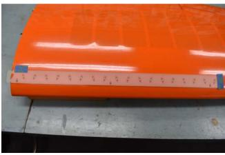
**23.** Use an X-Acto knife first to slice the covering and balsa sheeting down the center of the rectangular slots. Slice all the way through the thickness of the skin. Then use and insert the piercing tool. Do this for all the locations on the template.
