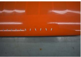
**28.** Move the template over as shown on STEP 7 on the drawing. The open end sits onto the last glued vortex generator. Repeat steps 23 through 26 for these last five vortex generators.
