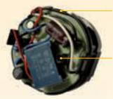
Integrated electronic and power supply board
