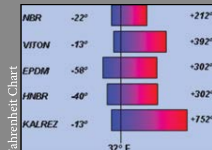
Maxium and Minimum admissible working temperature for O-Rings
