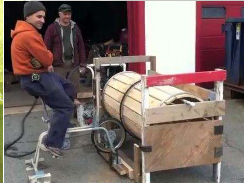
Open tech for farms: pedal-powered root washer. Credit: farmhack.net
