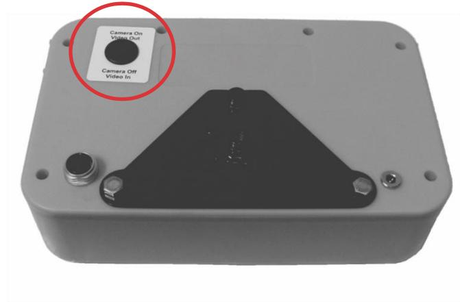
Note: with camera on and external signal coming into the front panel, the 2 signals will combine and give a distorted image on the LCD.
