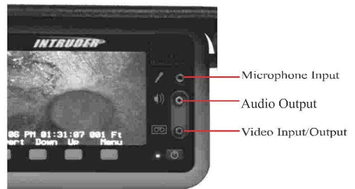
Connect audio out jack of the DrainCam display (indicated by speaker symbol) to audio input of recording device using a standard RCA audio cable.
