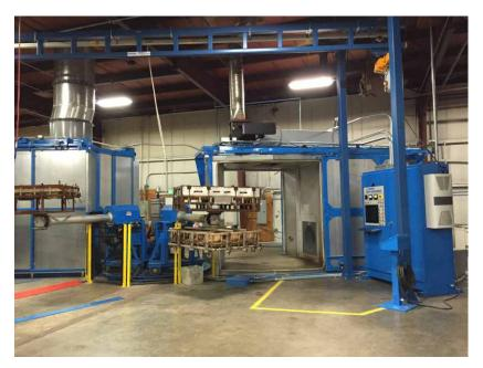
Jeco pallets are rotationally molded using 100% pure virgin LLDPE.
