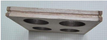
Slot Cut for Elevator Wire
