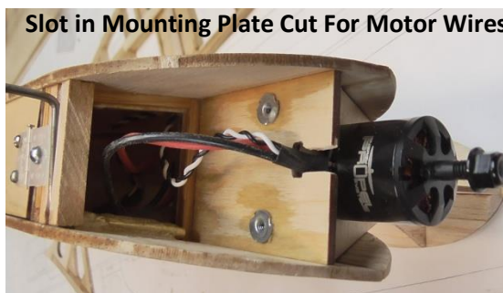
Depending on Motor orientation, wires may be run over the top and then down through the mount base
