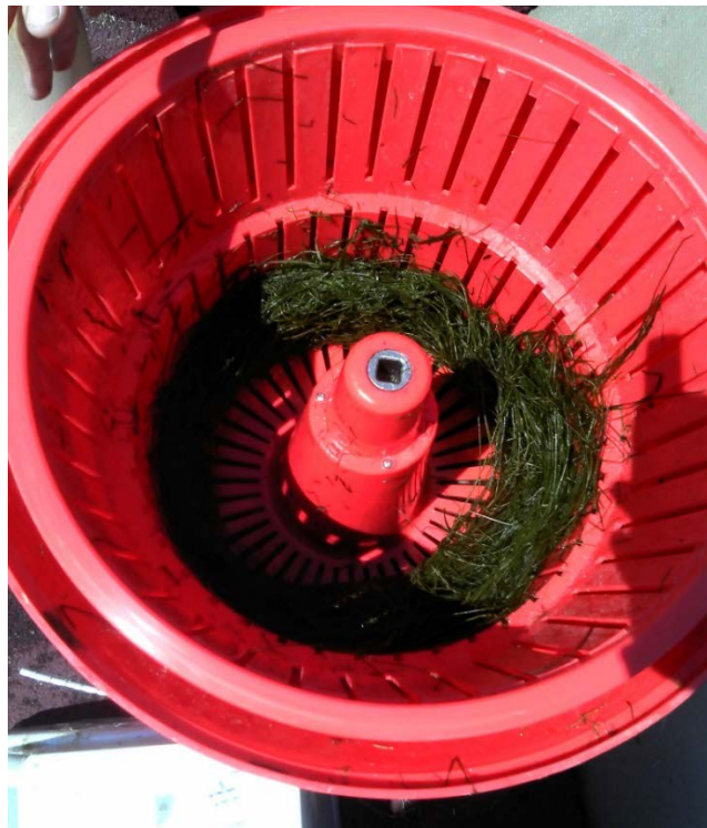
Figure 4- Commercial salad spinner used to spin starry stonewort before its wet weight measurement.
